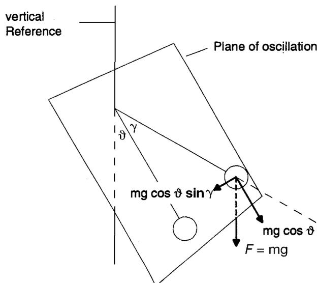
Fig. 6: Analysis of forces for a pendulum with inclined plane of oscillation (g pendulum).
