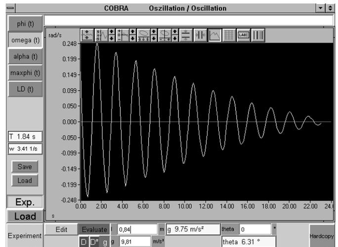
(ASCII File Data). The following measurement values are found in the single columns:  $t$  / (s) running time,  $\varphi(t)$  / (rad) angle,  $\omega(t)$  / (rad/s) angular velocity,  $\alpha(t)$  / (rad/s<sup>2</sup>) angular acceleration,  $\text{maxphi}(t)$  / (rad) positive peaks of the angle graph,  $T$  / (s) oscillation period.
